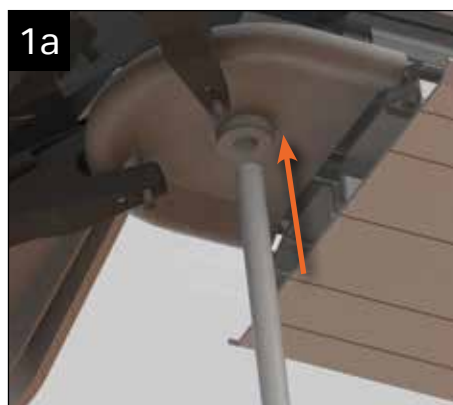
1a Tie bar at finial Insert the tie steel rod thread into the base of the spider. Measure the drop of the rod and cut to suit the position or the tie bar boss ring.
